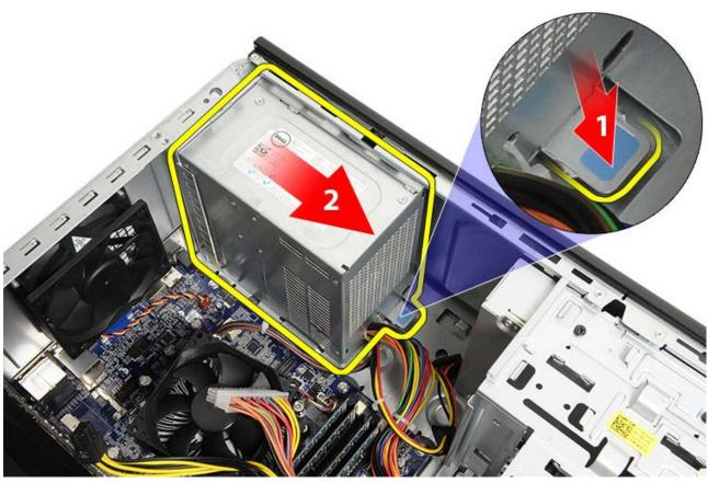
9. Lift the power supply out of the computer.
