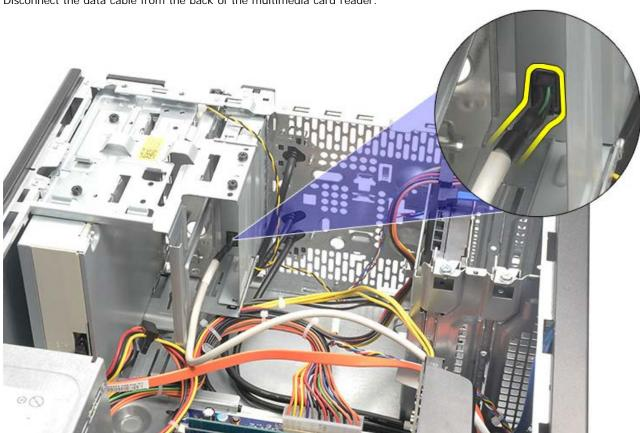
7. Remove the two screws that secure the multimedia card reader to the drive cage.
