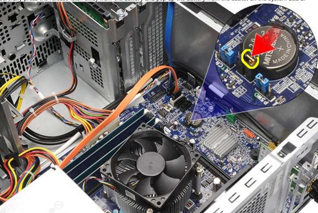
6. Lift the coin-cell battery out of the computer.
