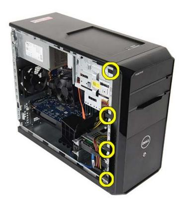
4. Rotate the bezel away from the computer to release the hooks on the opposite edge of the bezel from the chassis.
