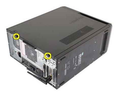
3. Slide the computer cover towards the back of the computer, and then remove it from the computer.
