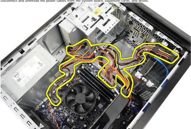
5. Disengage the cables from the routing clips, if present, on the computer.
