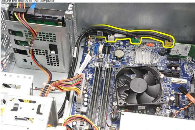
7. Remove the two screws that secure the front I/O panel to the computer.
