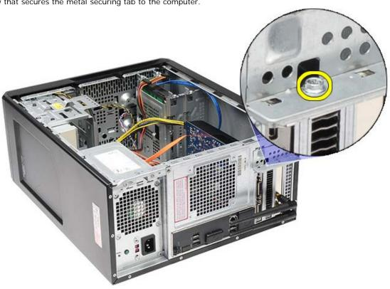
5. Remove the metal securing tab away from the computer.
