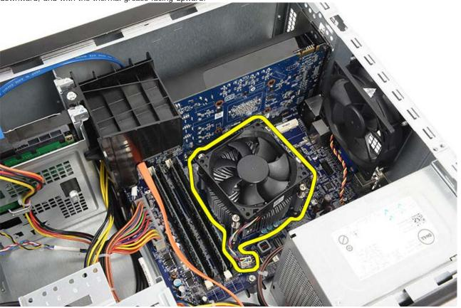
6. Push the release lever down and then press it outward to release it from the retention hook that secures it.
