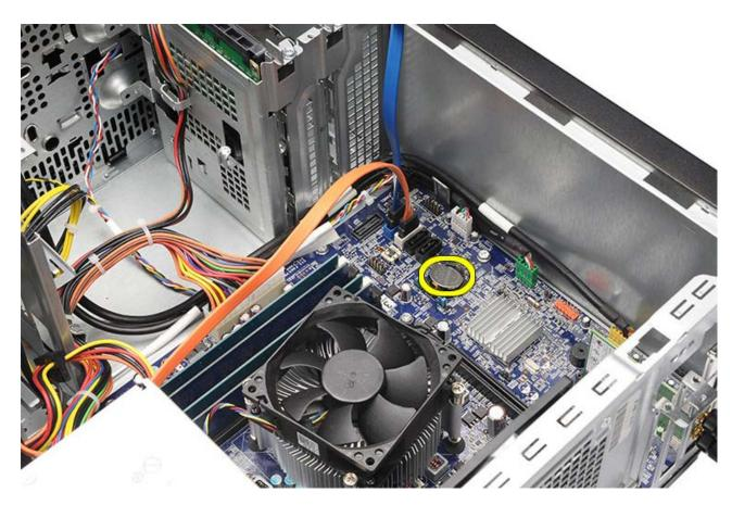
Related tasks Installing Coin-Cell Battery
