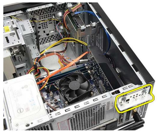
6. Disconnect the cables that are connected to the video card.
