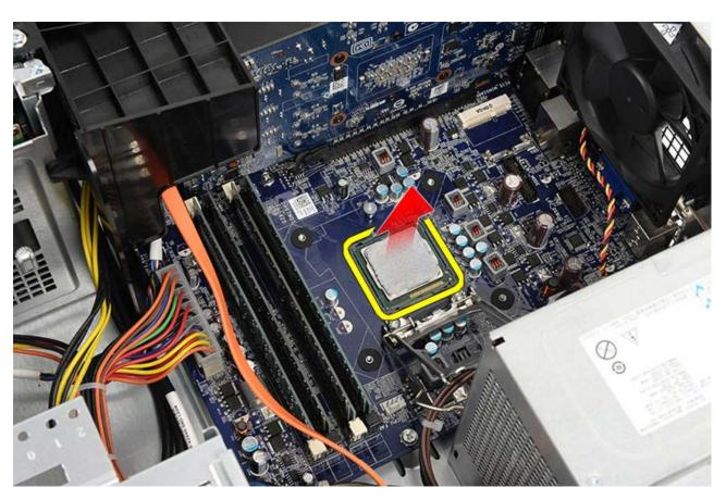
Related tasks Installing Processor
