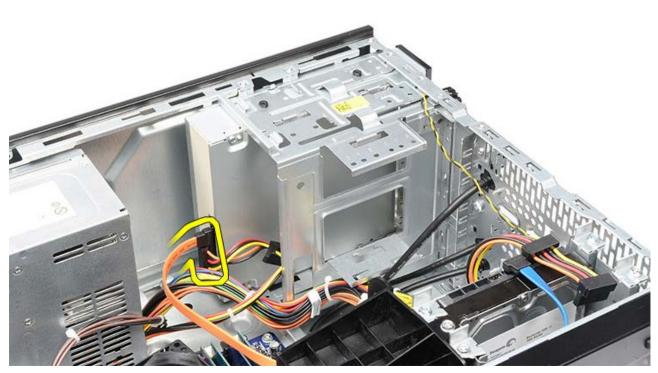
5. Remove the screws that secure the optical drive to the drive cage.
