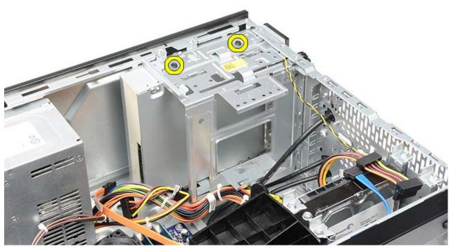
6. Slide out the optical drive through the front of the computer.
